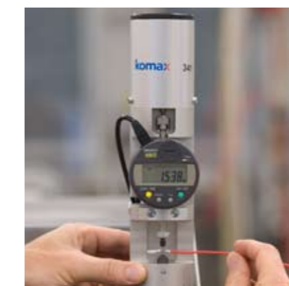
Komax 341 crimp height measuring device
