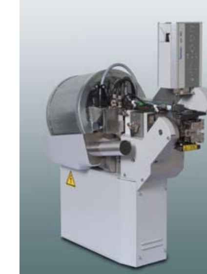
mci 765 seal loading module with seal position monitoring (SPM)
