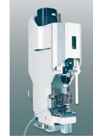
mci 722 crimping module with programmable crimp height
