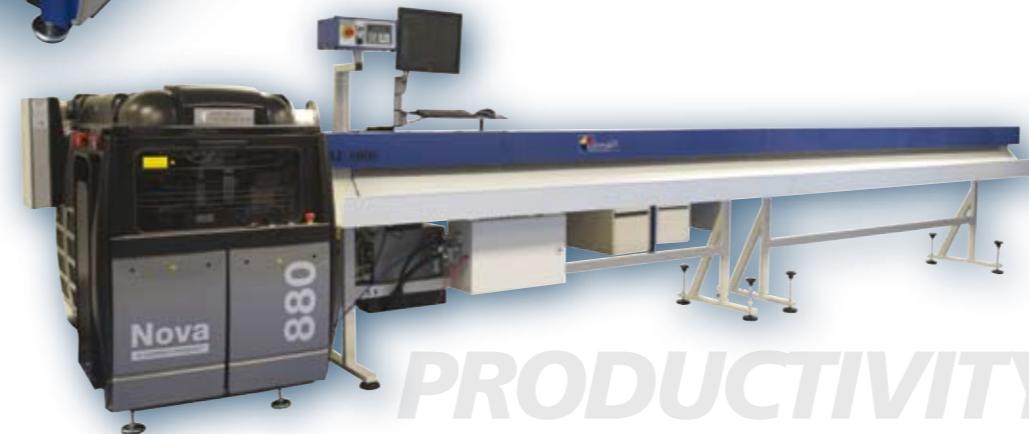
Above: Automated Nova 880 with ASL pre-loaded with 32 wires for faster processing and changeover
