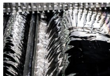
Stable solder wave height up to 16 mm possible
