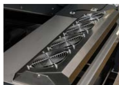
Efficient cooling in outfeed section
