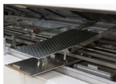
Retractable nozzle sheets for quick maintenance
