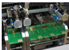
Multi track conveyor for variable PCB width
